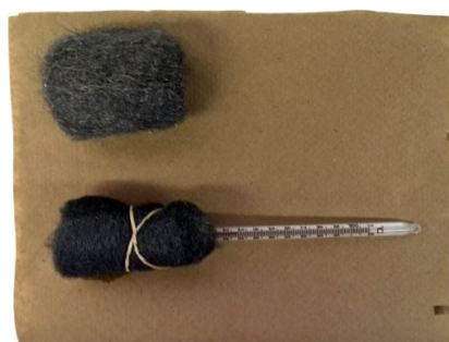
Figure 4. Thermometer wrapped with vinegar-treated steel wool
