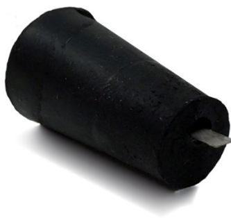
Figure 5. Magnesium ribbon inserted into the rubber stopper
